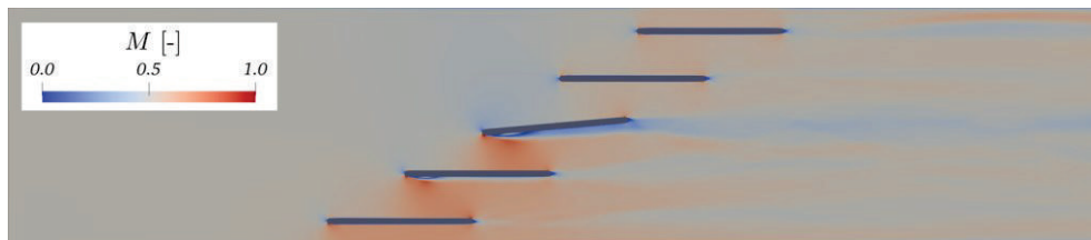
Fig. 8. Field of Mach number obtained from time-averaged velocity fields, Nektar++, incompressible simulation.
