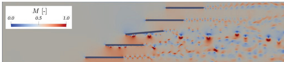
Fig. 7. Instant field of Mach number from incompressible simulation of Nektar++ illustrates small vortical structures.
