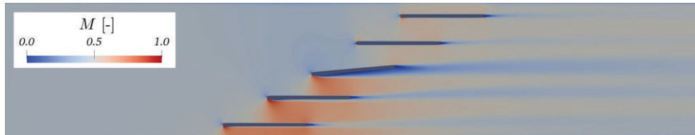
Fig. 6. Mach number distribution from OpenFOAM simulation ( LU-SGS, \gamma -SST ) for \alpha = -5^\circ .
